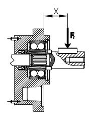
X = Distance of the radial flange result from the mounting flange
